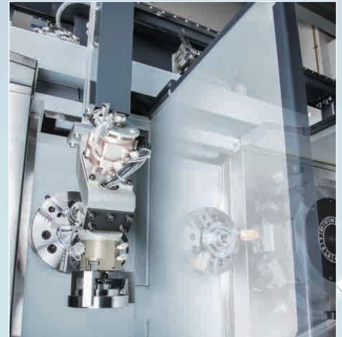
2 1st spindle unloading / loading
